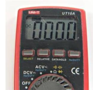
It may seem strange to have zero when the button is pressed and have 5 volts when it is released. This is called "active low", because the signal is low when the condition is happening. Active low signals are very common practice in electronics, especially for pushbuttons.
