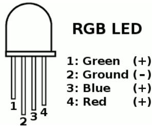
You will need to spread the pins slightly so they fit into 4 separate groups of holes. Pin 2 needs to be connected to ground, so place a short wire between that hole group and the ground row.
